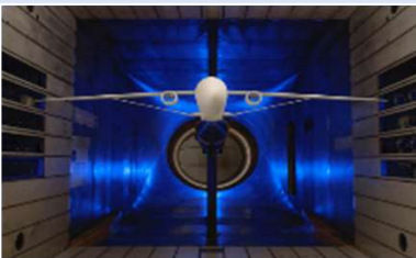
Transonic Truss-Braced Wing 5-10% fuel burn benefit
